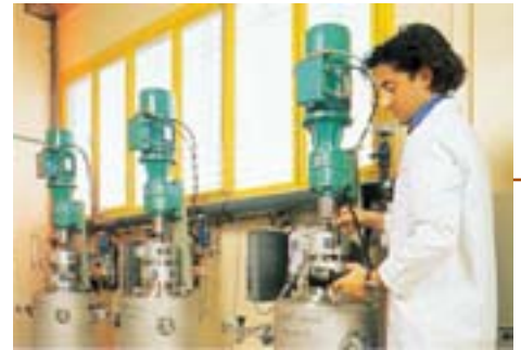
Test platform for development of a customer-specific rotary shaft sealing system
