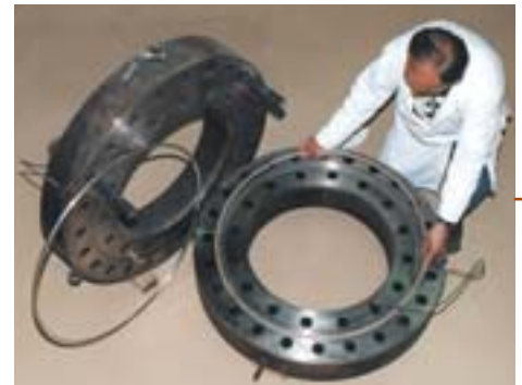
Test platform for checking behaviour of Light Water Reactor vessel seal against flange surface defects
