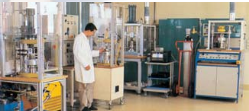
Test stands for cycling at pressure and temperature : valve rising stems and 1/4-turn stems, and poppet valve seats
