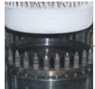
Testing of 820mm piston seal in graphite material (800°C, slow-motion)
