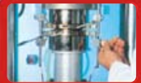
Heated platens for seal characterization at temperature
